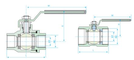
QL11F内螺纹连接二片式球阀 QL11F female threaded two pieces ball valve
