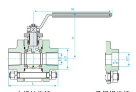
内螺纹连接 Female threaded connection
